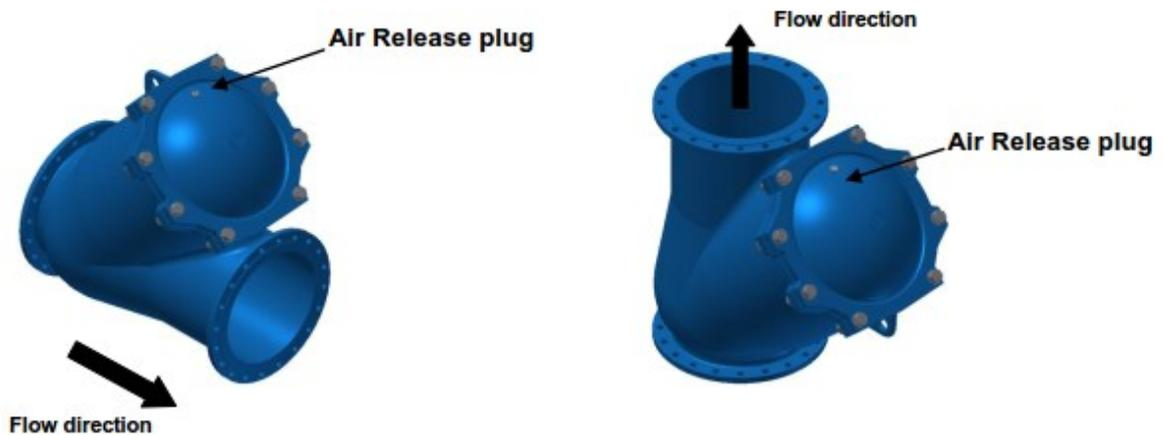
To eliminate the air proceed by unscrewing the plug in order to release the accumulated air until the fluid is coming out. The plug is auto blocked and cannot be unscrewed totally. If the plug is damaged or blocked, proceed disassembly of the bonnet as indicated in previous content. It is recommended to clean the plug when bonnet is disassembled for maintenance.
