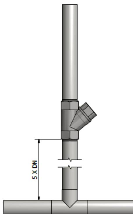
Fig. 3256 Vertical Installation after bend
