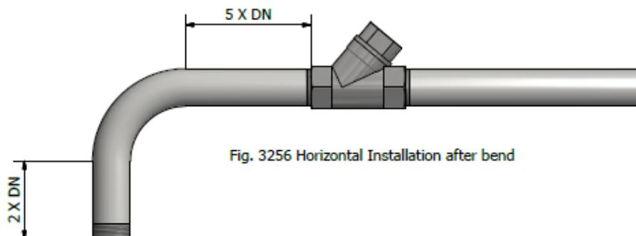
Fig. 3256 Horizontal Installation after bend
