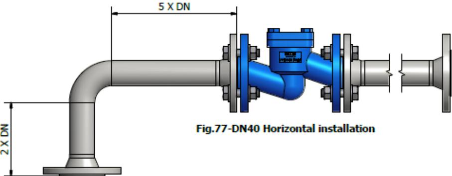
Fig.77-DN40 Horizontal installation
