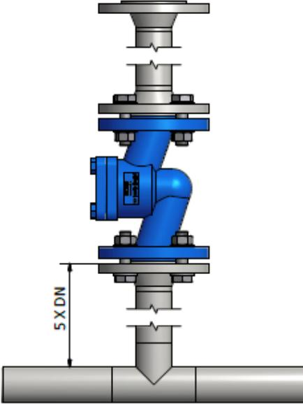
Fig.77-DN40 Vertical installation after bend
