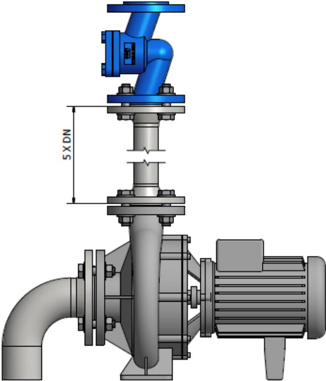
Fig.77-DN40 Vertical installation after pump
