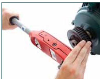
TIGHTEN SCREWS TO THE CORRECT TORQUE SETTING
