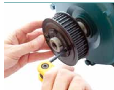
TIGHTEN SCREWS ALTERNATELY
