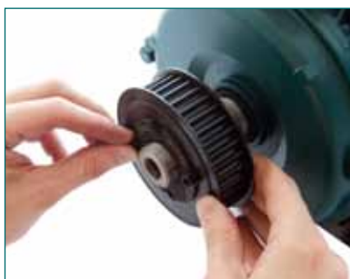
TIGHTEN SCREWS FINGER TIGHT
